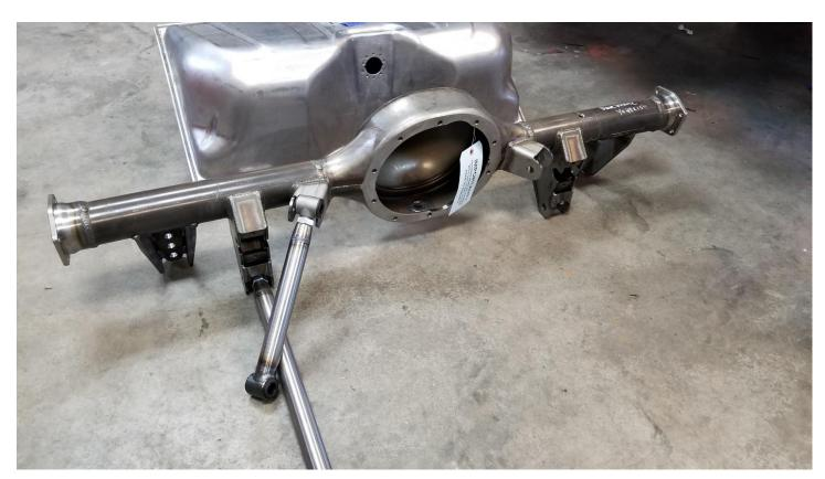
We started with a complete rear end housing that is designed for a Ford 9" inch third member. We also requested that all the brackets and shock mounts be welded in place. This is the easiest approach to installation since the factory has already calculated the necessary angles and locations. If you're going to reuse an existing rear end, you'll have to weld all the brackets to the axle housing.
