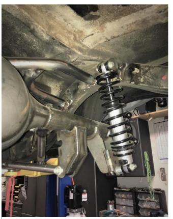
Once everything is welded into place you can lower your car and adjust the ride height using the three different lower shock mounting locations. You can verily the spring height a bit, but do not use it as the primary adjustment for ride height.
