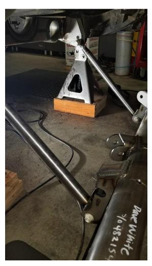
Use the flap wheel on the grinder and remove all undercoating, paint or debris that has accumulated. Use a solvent or cleaning agent to remove as much as possible to avoid contamination. Go back over the area again with a fresh flap wheel to make sure you get clean bare metal.
