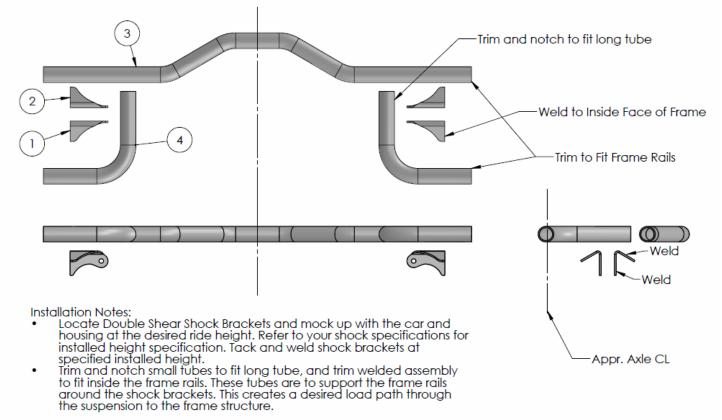
The rear crossmember does not have any specific measurements or geometric reference because it's simply there as added support and provides torsional rigidity (\*see note above). You can weld it in based up the photo on the opening page or the included photo shown below.
