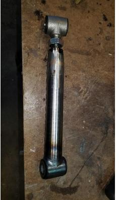
The challenge at this point is to try and maintain your angles called out on sheet 3 from above. The lower bars should be from **0d to -.05D**, the upper bars should be between **0.5 -1.5d** and the axle housing face should be **90d**.
