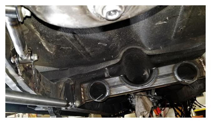
Once the upper bars are tacked into place, assemble and install the rear shocks and mounting tabs onto the lower shock mount. Grind away any existing frame undercoating or paint and prepare for welding. The upper shock mount location is undefined in terms of geometry, make sure the angle of the shock
