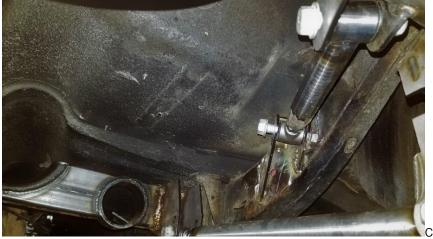
springs provides sufficient clearance to clear the bracket.
