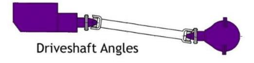
Record the angle as "3 degrees up" or "2 degrees down, etc. Next, measure the transmission and differential angles, locate a machined surface on the
